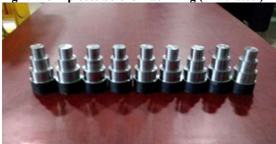
Fig 3. Work pieces after machining (EN19 Steel)
