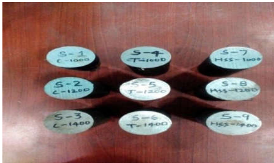
Fig 2. Work pieces before machining (EN19 steel)
